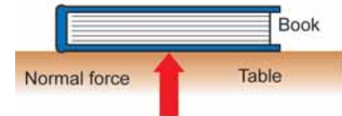
Figure 13.16: The normal force and the weight are equal in strength and opposite in direction.
