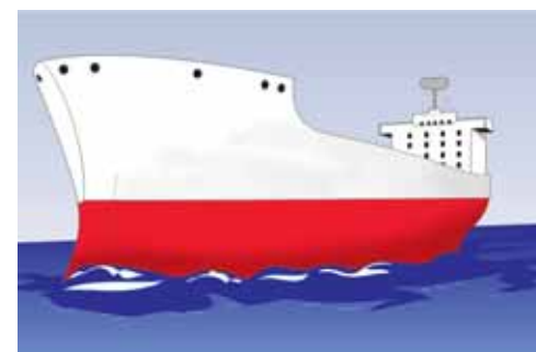
Empty cargo ship - less displaced water
